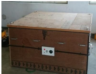
**Fig 3 HACC (Hot Air Curing Chamber-2013, Source: Concrete lab equipment, JIT)**
